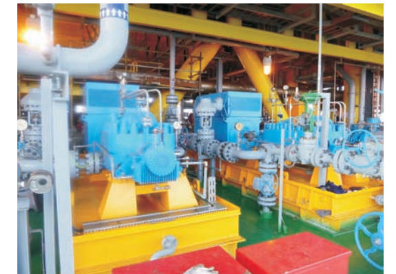
中海油湛江涠洲12-2/11-4N油田海上平台注水泵 CNOOC Zhanjiang Weizhou 12-2/11-4N oilfield offshore water injection pump KDY100-150*8(Q=100M 3 /H,H=1480m n=3300rpm)
